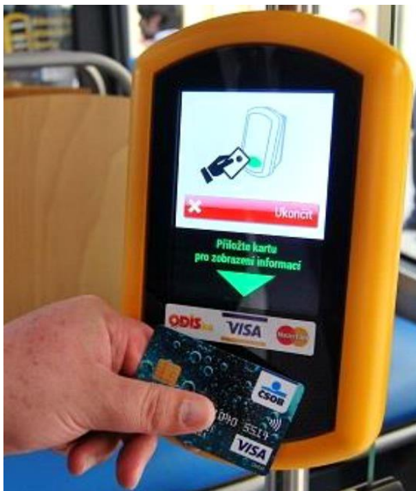
Figure 4.4.9: Terminal in DPO vehicles – card enclosure when exiting (see http://www.buspress.eu/ostrava-spousti-nejmodernejsi-evropsky-system-placeni-v-mhd/ )
