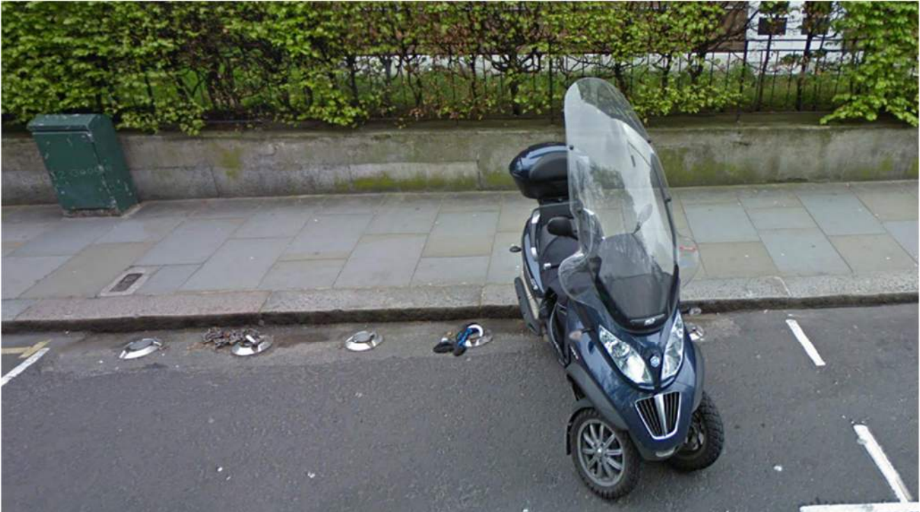
Photo 3.5 – On street anchor points, allow 6 motorcycles within a standard car parking bay
